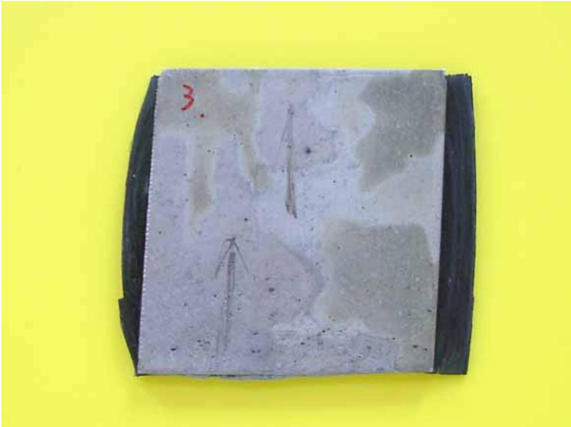
Fig. 3.3 Mg/APC-2 laminate with 4 plies of APC-2 prepreg sandwiched by two AZ31 Mg sheets formed at 400°C under 0.7 MPa (sample 3 in Table 3.1).
