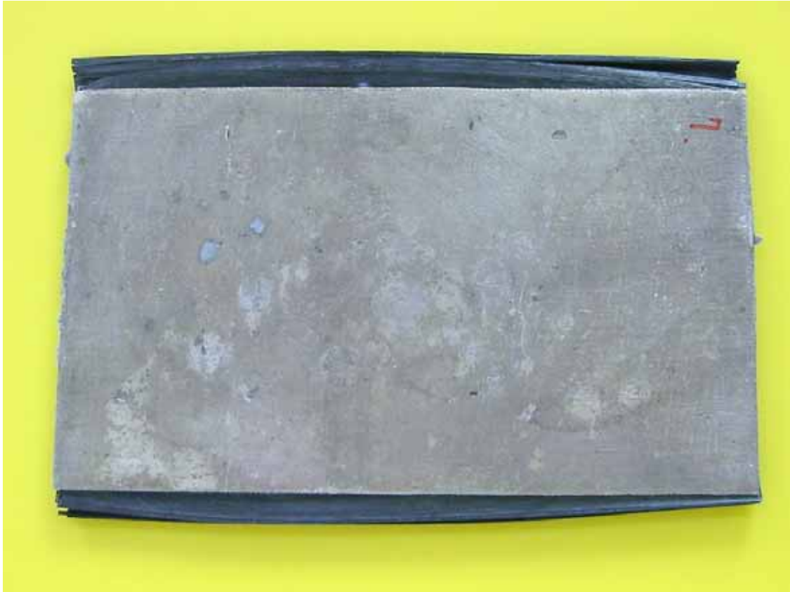
Fig. 3.7 Mg/APC-2 laminate with 2 plies of APC-2 prepreg each layer and laminated in the stacking sequence of Mg/ APC-2/Mg/APC-2/Mg formed at 400°C under 1.4 MPa (sample 7 in Table 3.1).
