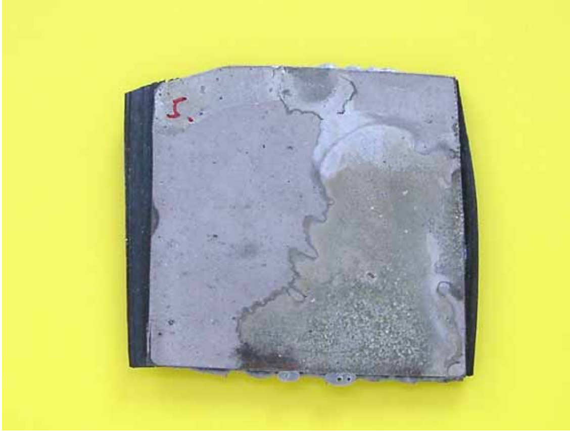
Fig. 3.5 Mg/APC-2 laminate with 3 plies of APC-2 prepreg sandwiched by two AZ31 Mg sheets formed at 400°C under 1.0 MPa (sample 5 in Table 3.1).
