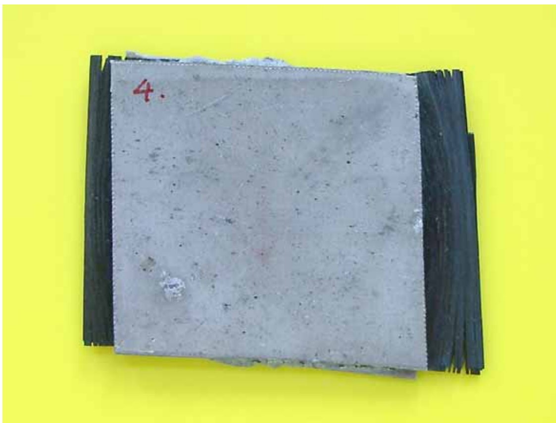
Fig. 3.4 Mg/APC-2 laminate with 4 plies of APC-2 prepreg sandwiched by two AZ31 Mg sheets formed at 400 °C under 1.6 MPa (sample 4 in Table 3.1).
