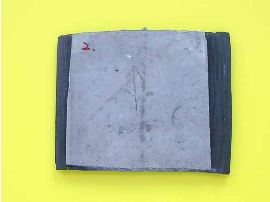
Fig. 3.2 Mg/APC-2 laminate with 4 plies of APC-2 prepreg sandwiched by two AZ31 Mg sheets formed at 400°C under 0.7 MPa (sample 2 in Table 3.1).
