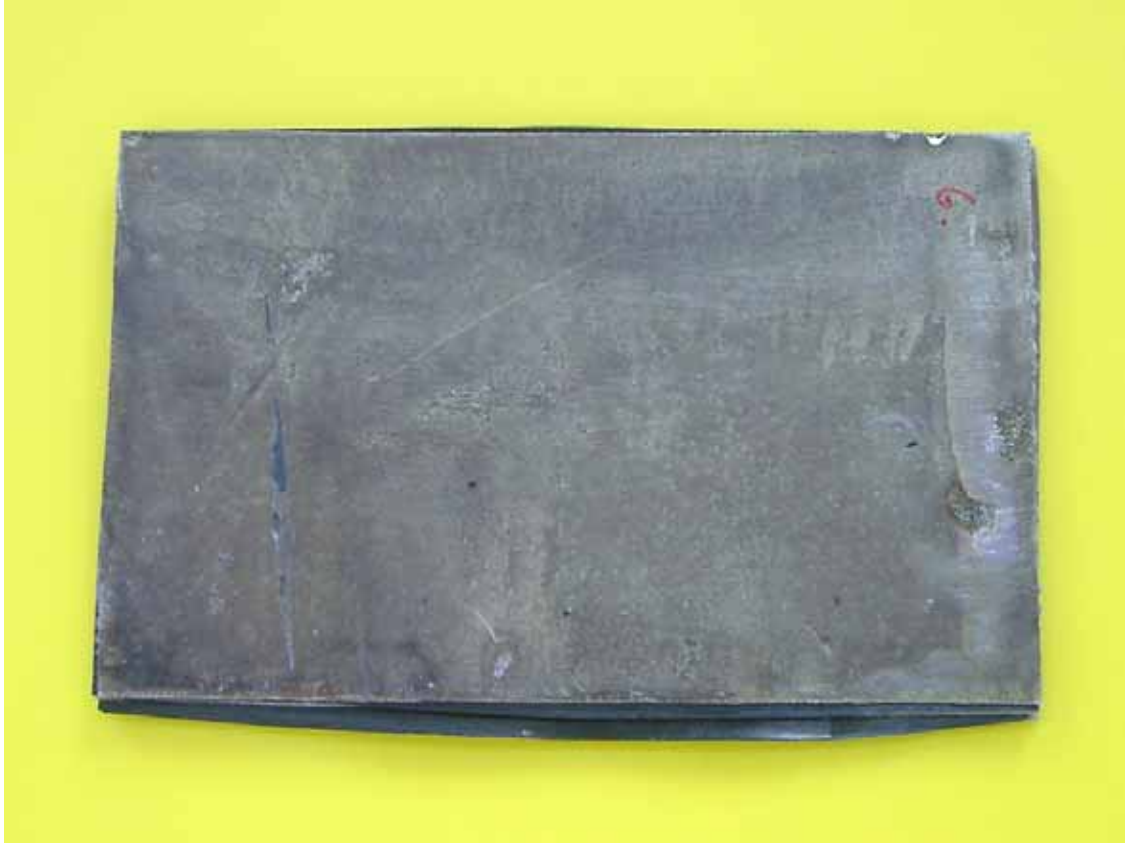
Fig. 3.6 Mg/APC-2 laminate with 2 plies of APC-2 prepreg each layer and laminated in the stacking sequence of Mg/ APC-2/Mg/APC-2/Mg formed at 400°C under 0.7 MPa (sample 6 in Table 3.1).
